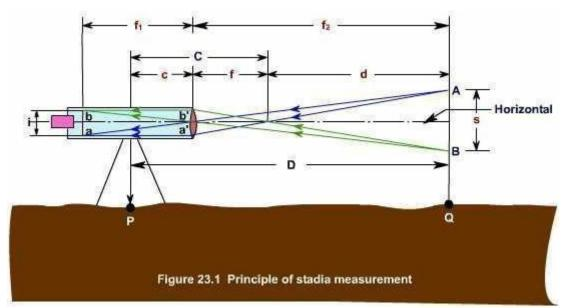
By the laws of optics, the images of readings at A and B of the staff will appear along the stadia hairs at a and b respectively. Let the staff interval i.e., the difference between the readings at A and B be designated by s. Similar triangle between the object and image will form with vertex at the focus of the objective lens (F). Let the ho rizontal distance of the staff from F be d. Then, from the similar Ds ABF and a' b' F,
